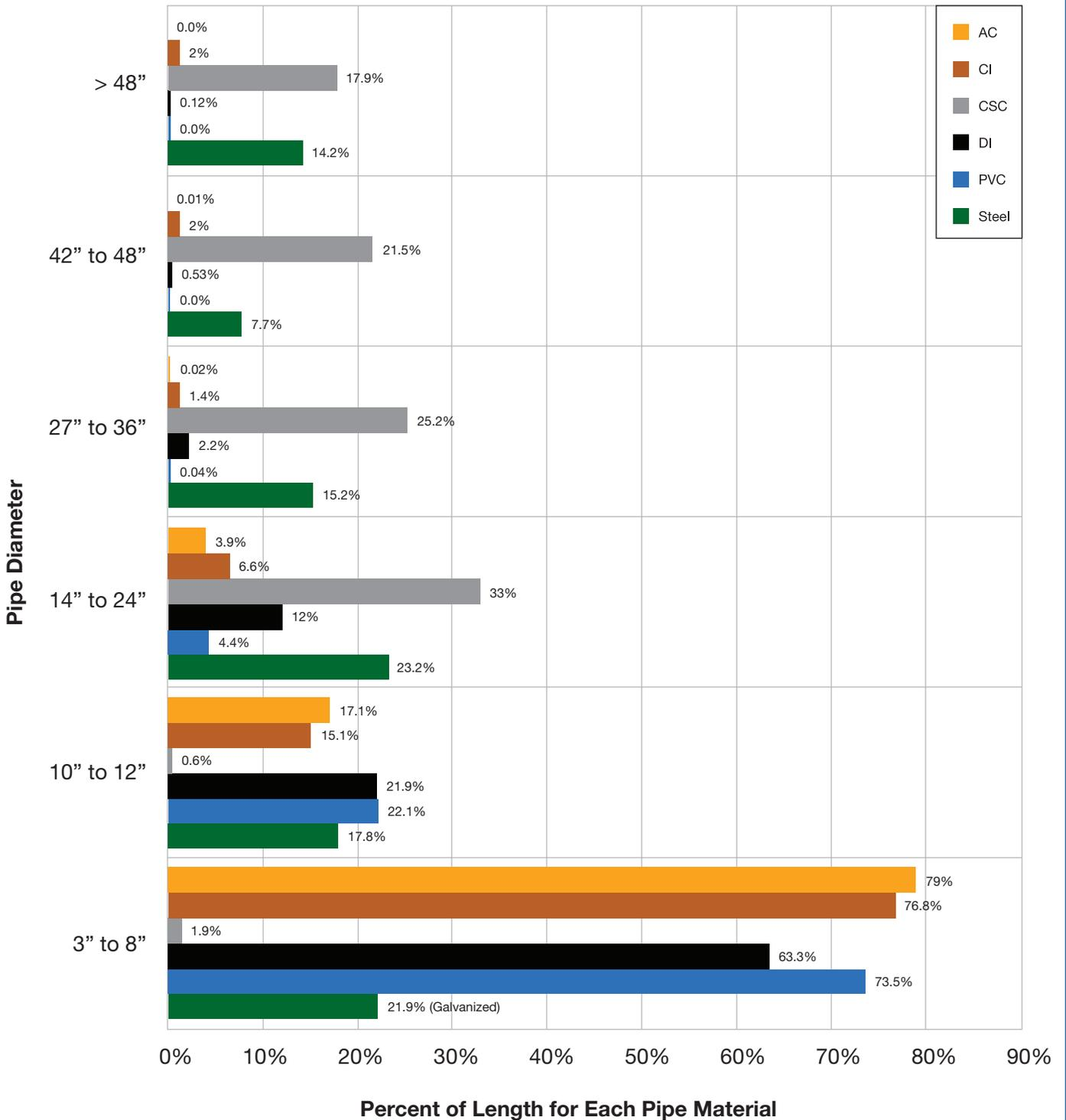
**FIGURE 17: PERCENT OF TOTAL PIPE LENGTH BROKEN DOWN BY PIPE DIAMETER AND MATERIAL TYPE FROM THE DETAILED SURVEY**
