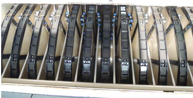
Figure 48: Schematic of a disc filter
