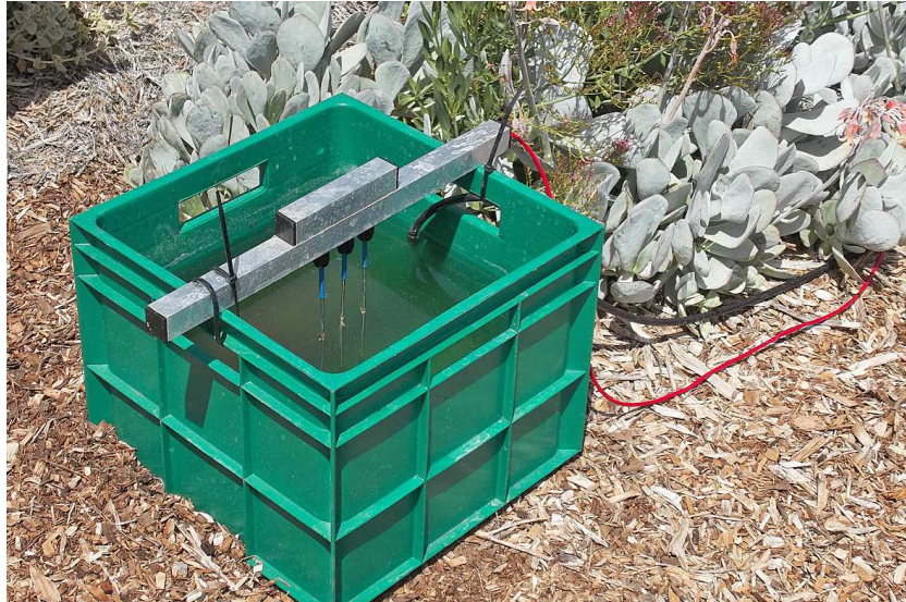
Level sensor resting on the evaporator
