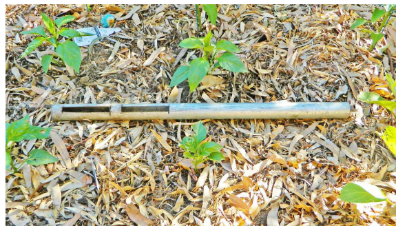
An angle grinder can be used to make some slots in a length of steel pipe
