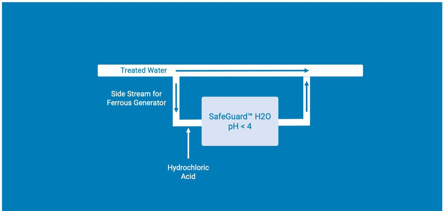
SafeGuard™ H2O Arsenic Removal Technology Schematic
