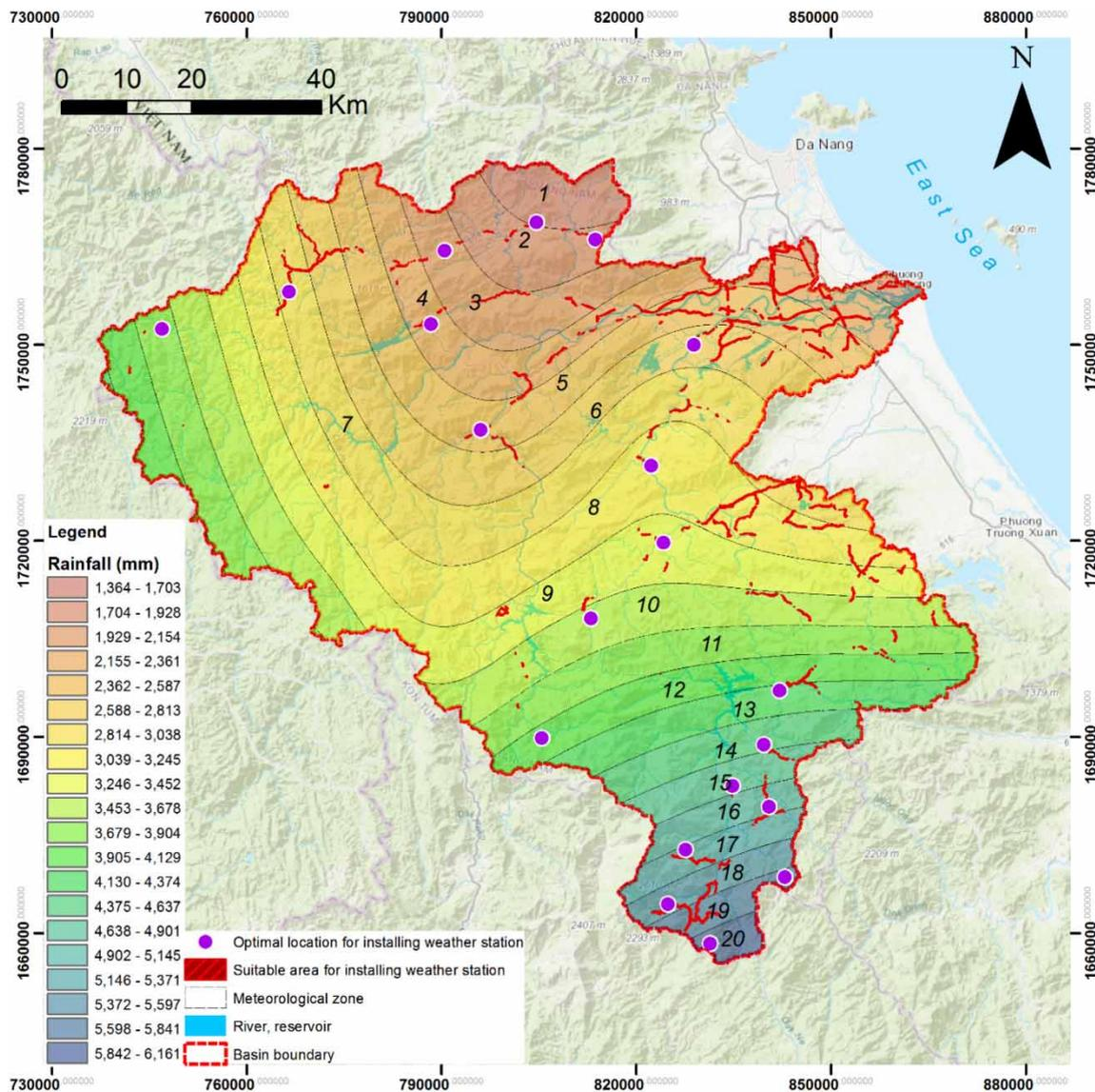
Figure 7 | The suitable areas and optimal locations for installing weather stations on VGTB river basin.
