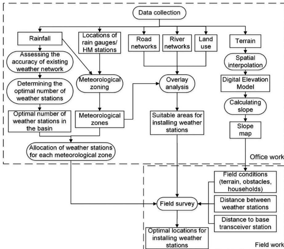
Figure 4 | The process for optimizing meteorological network on VGTB river basin.
