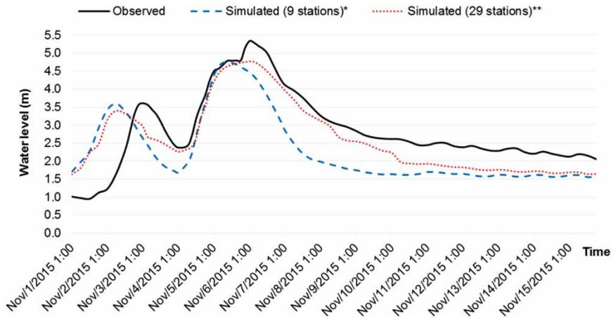
**Figure 14** | Comparisons between observed and simulated water levels on hourly timestep at Giao Thuy stream gauge during flood events in November 2015. (\*nine rain gauges, HM stations operated by Mid-Central Hydro-Meteorological Centre; \*\*nine rain gauges, HM stations operated by Mid-Central Hydro-Meteorological Centre plus 20 automatic weather stations).
