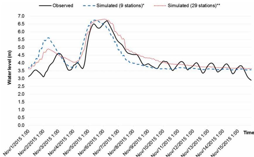
**Figure 13** | Comparisons between observed and simulated water levels on hourly timestep at Ai Nghia stream gauge during flood events in November 2015. (\*nine rain gauges, HM stations operated by Mid-Central Hydro-Meteorological Centre; \*\*nine rain gauges, HM stations operated by Mid-Central Hydro-Meteorological Centre plus 20 automatic weather stations).
