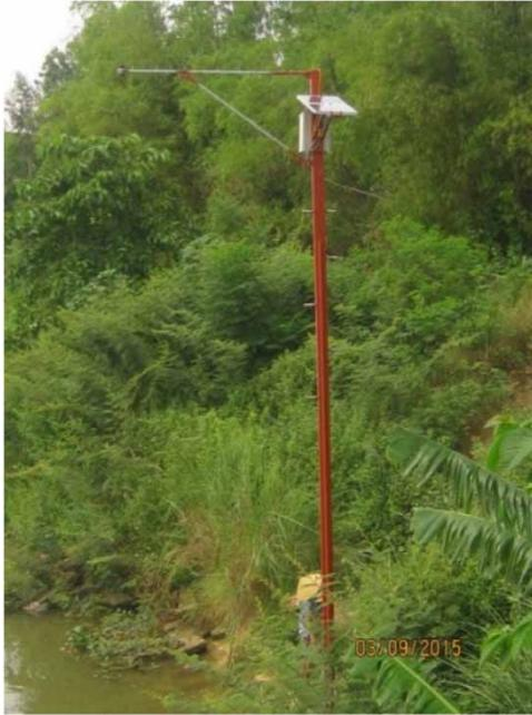
**Figure 10** | Automatic hydrological station installed on VGTB river basin. Photograph taken by authors.
