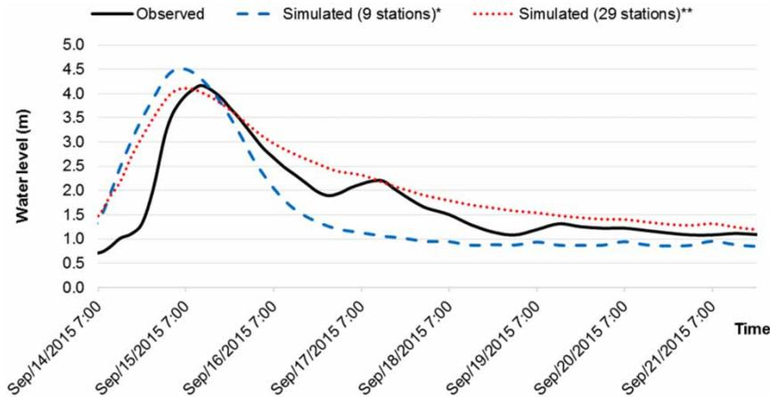
**Figure 12** | Comparisons between observed and simulated water levels on hourly timestep at Giau Thuy stream gauge during flood event in September 2015. (\*nine rain gauges, HM stations operated by Mid-Central Hydro-Meteorological Centre; \*\*nine rain gauges, HM stations operated by Mid-Central Hydro-Meteorological Centre plus 20 automatic weather stations).
