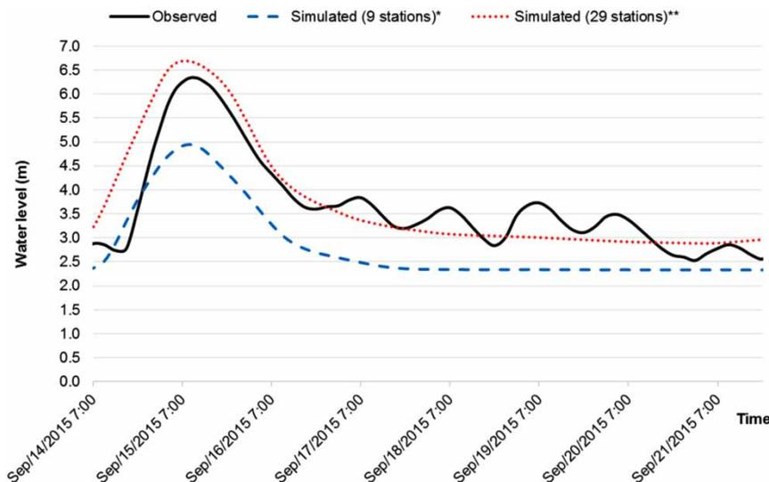
**Figure 11** | Comparisons between observed and simulated water levels on hourly timestep at Ai Nghia stream gauge during a flood event in September 2015. (\*nine rain gauges, HM stations operated by Mid-Central Hydro-Meteorological Centre; \*\*nine rain gauges, HM stations operated by Mid-Central Hydro-Meteorological Centre plus 20 automatic weather stations).
