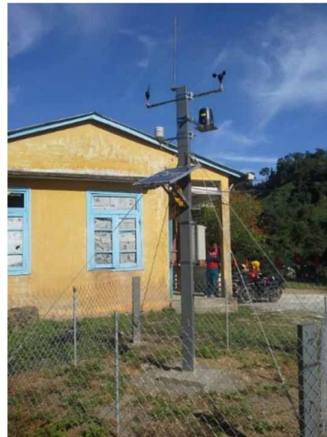
**Figure 8** | Automatic weather station installed on VGTB river basin. Photograph taken by authors.
