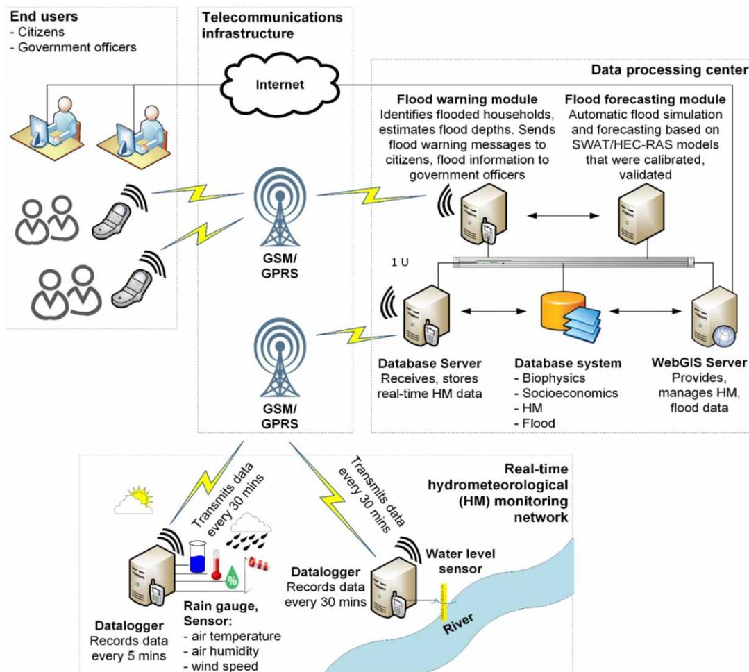
Figure 3 | The structure of real-time flood early warning system in VGTB river basin (Nguyen et al. 2020).
