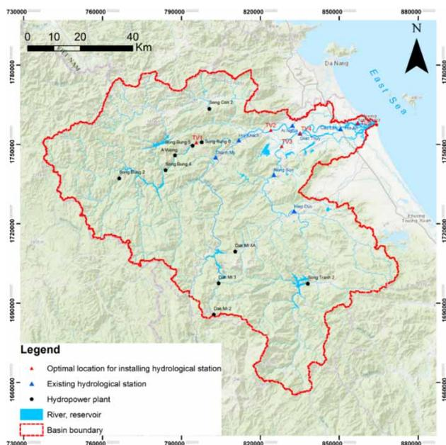
Figure 9 | The optimal locations for installing hydrological stations on VGTB river basin.
