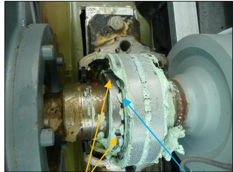
Multiple notches on the clamping ring will allow to insert the tab in the best position
