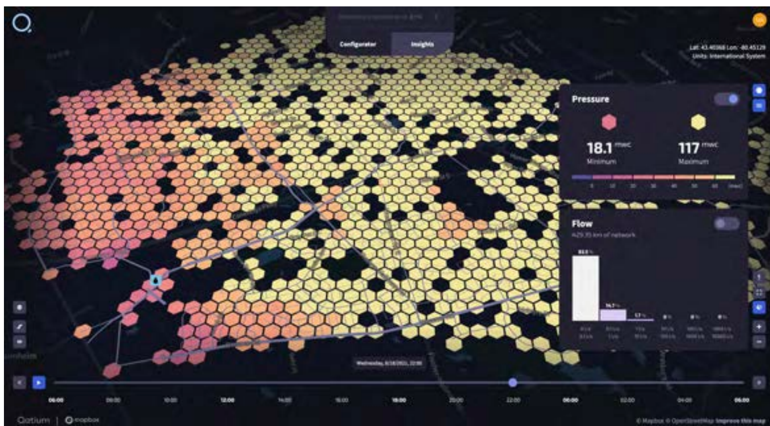
Visualization layer showing variation of available pressure within the network
