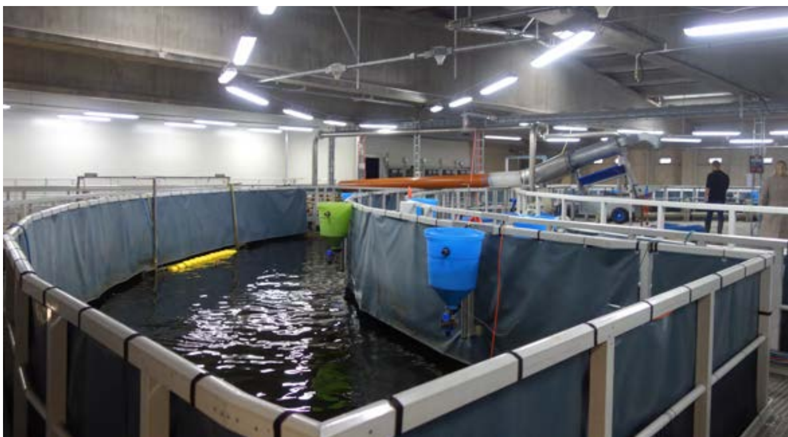
The recirculating system, the RAS 2020 with a diameter of 32 meters and a depth of 4.5 meters holds 2,700 cubic meters of water.
