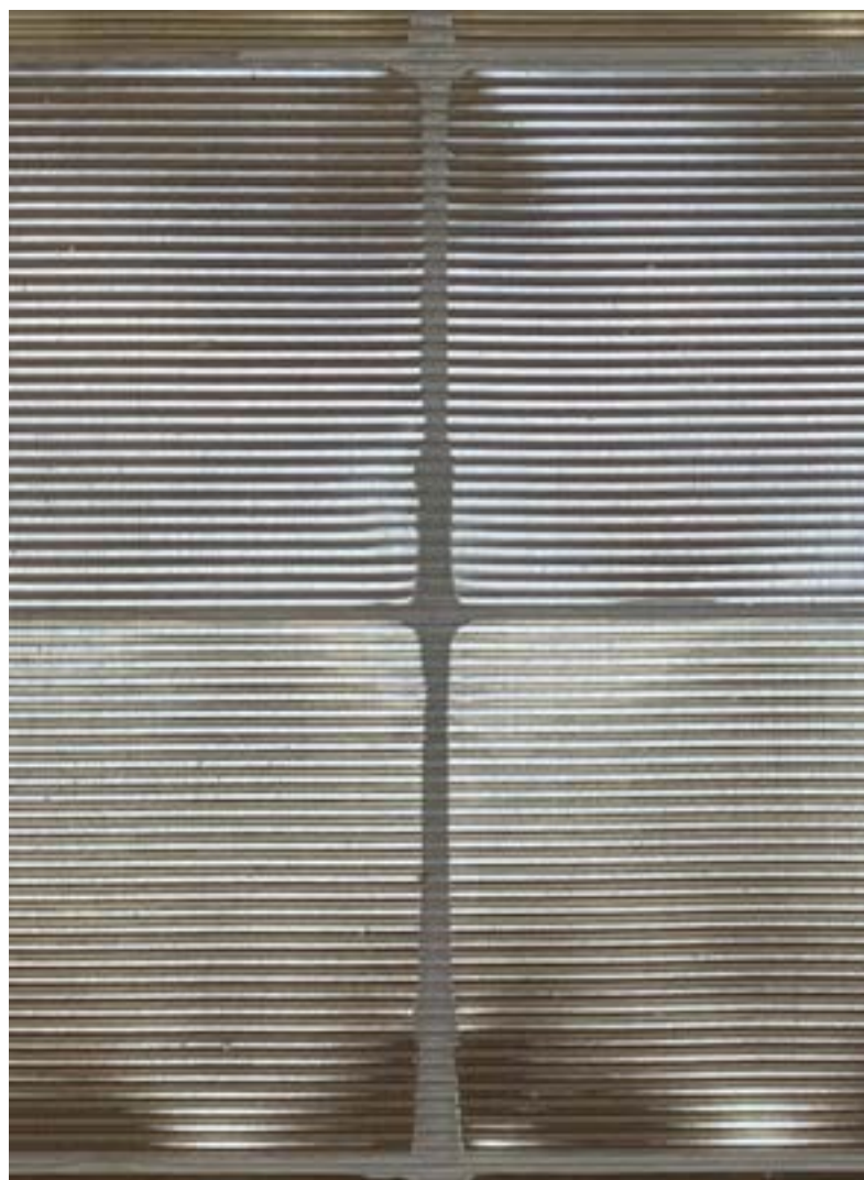
The construction of the filter panels from GKD with shovel-like support structure, consisting of many small squares of mesh connected with one another, augments the filter effect.
