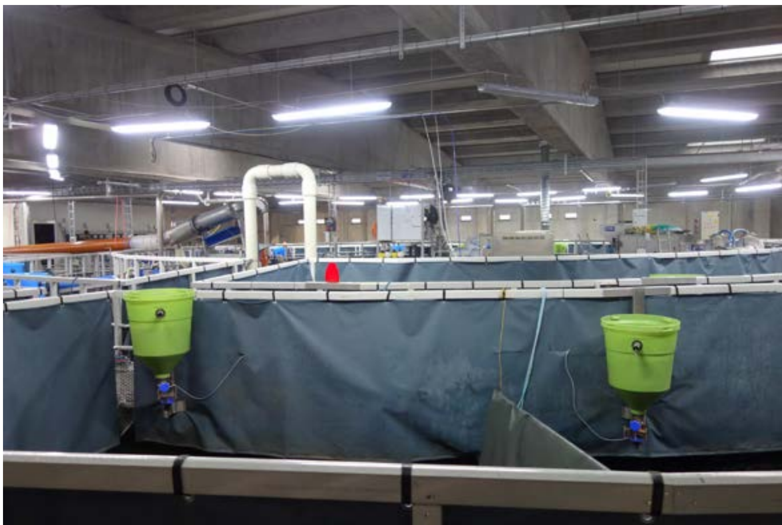
The core element of the farm at Swiss Alpine Fish is the innovative RAS 2020 recirculating system.
