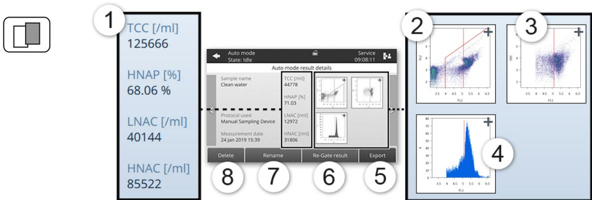
Figure 2 - 1 : Display of a single measurement result, using a TCC cartridge
