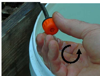
5. If your plants are getting too much water, turn the control dripper anticlockwise to increase the flow rate of the control dripper.
