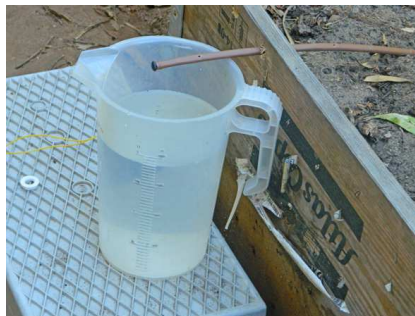
Dripper control volume in measuring container
