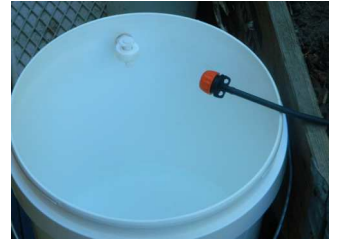
The adjustable drip drips water into the evaporator during irrigation
