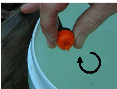
4. If your plants are getting too little water, turn the control dripper clockwise to reduce the flow rate of the control dripper.
