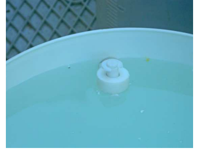
Water level just below the float switch
