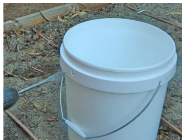
Drill a hole in the side of the evaporator
