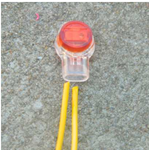
Wires are not stripped before insertion
