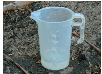
3. After sunrise the following morning, check the amount of water in the measuring container.
