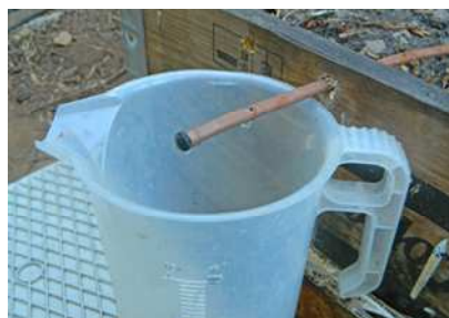
2. Position the measuring container under one of the irrigation drippers so that water drips into the container during the irrigation.
