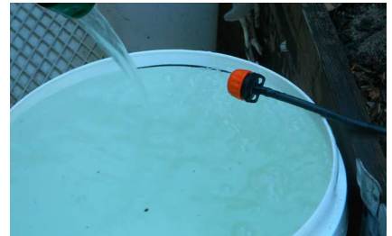
Fill the evaporator with water until the water level reaches the level line
