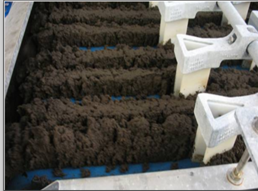
Biological Sludge blended with cationic polymer after ReXtract conditioning (shown on Belt Press)
