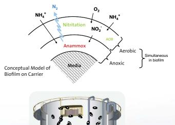
The ANITA Mox effluent screens provide a positive barrier to loss of anammox bacteria, since they keep the media and biofilm in the reactor.
