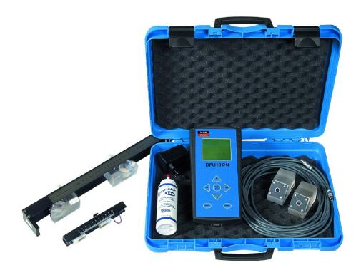
The FLT10 PN is an ultrasonic portable flowmeter for measurement of bidirectional flow in pressurized (full) pipes from ND 25mm up to 2000 mm. It provides high accurate measures without any insertion (tapping or drilling) by using external clamp on probes set (range from 2Mhz to 500Khz depending on size and pipes material)
