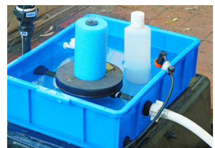
A full bottle of water decreases the surface area of evaporation
