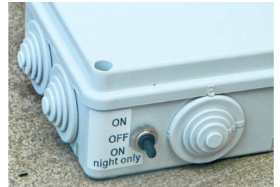
Switch with 3 positions: ON, OFF, ON night only
