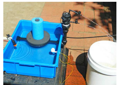
When the float reaches the high level the irrigation stops
