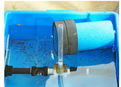
Remove the float to stop irrigating
