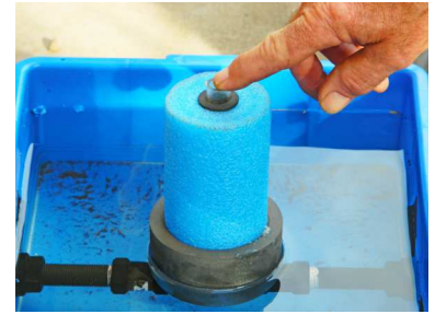
Push the float down to start irrigating
