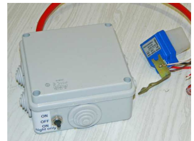
Waterproof control box and light sensor
