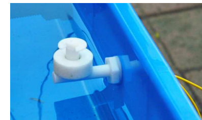
Irrigation starts automatically at the start time provided that the water level is below the float switch
