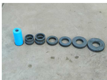
Cylindrical float and 8 float rings
