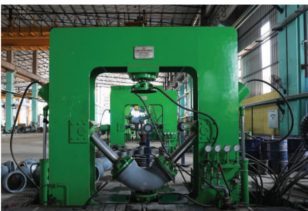
Hydrostatic Pressure Testing of Fittings
