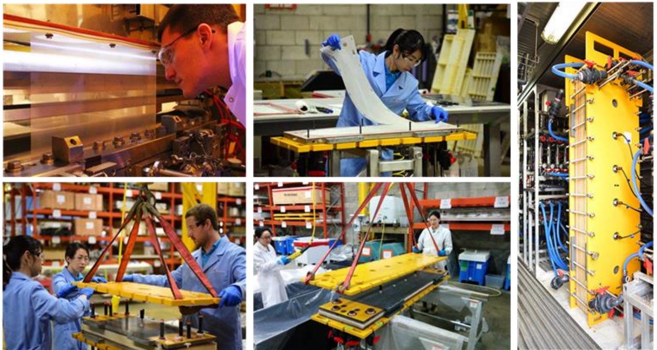
Figure 7. Full Scale Production of Electrodialysis Stacks
