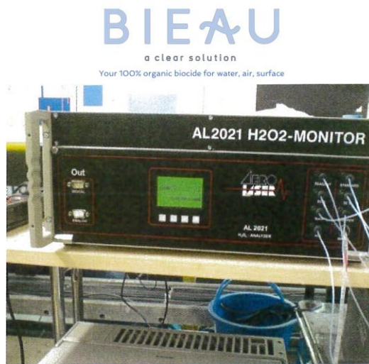
Figure 11: H 2 O 2 measurement using AeroLaser (optional)
