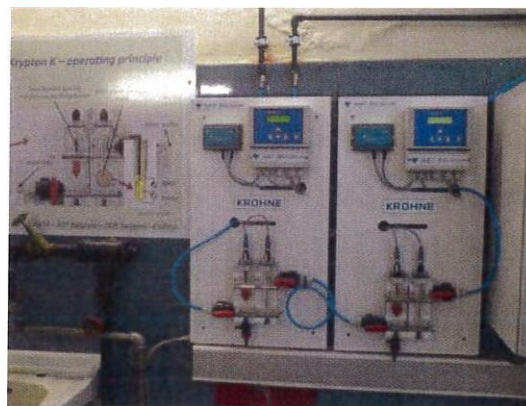
Figure 9: Measuring equipment Krypton K - Dr. A. Küntze (Kröhne).
