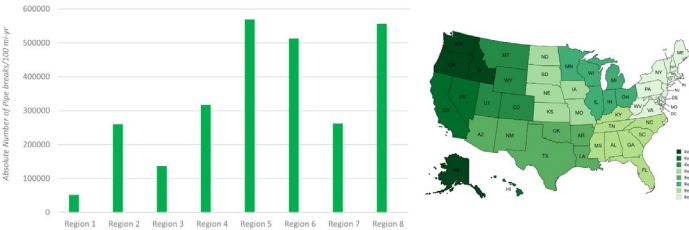
Exhibit 21. Absolute number of pipe breaks per US region. Data is weighted and scaled to arrive at nationwide figures. Dataset from Barfuss (2023).
