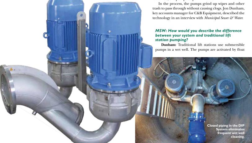
switches when the water reaches a preset level. The pumps then run at full speed to empty the wet well. In the DIP System, the inflow is piped directly into the pump — a wet well is not necessary. The pumps operate continuously and are controlled by a variable-frequency drive so they run at the speed necessary to handle the flow. It is not batch pumping.
