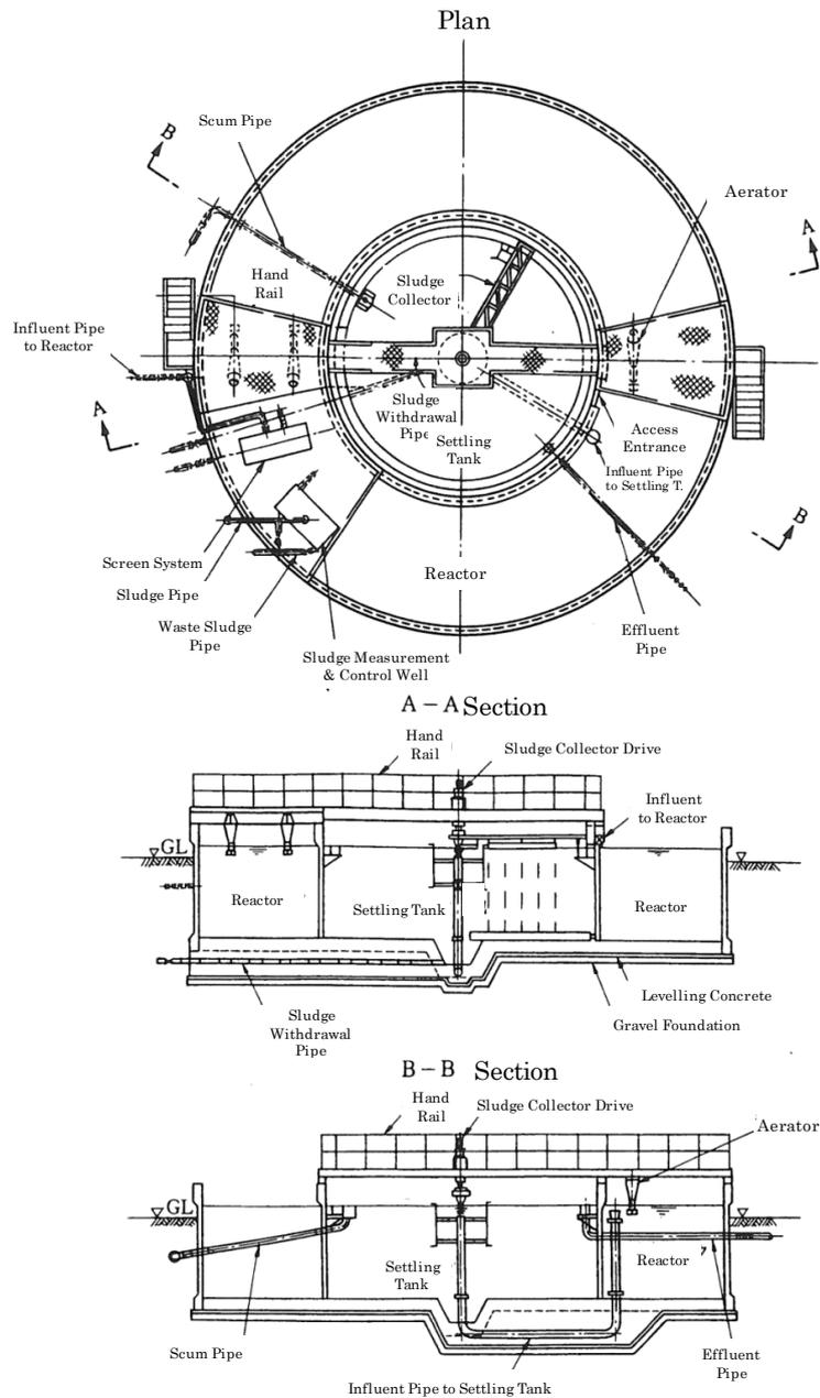
**Figure 5.20.2 Precast Oxidation Ditch**
