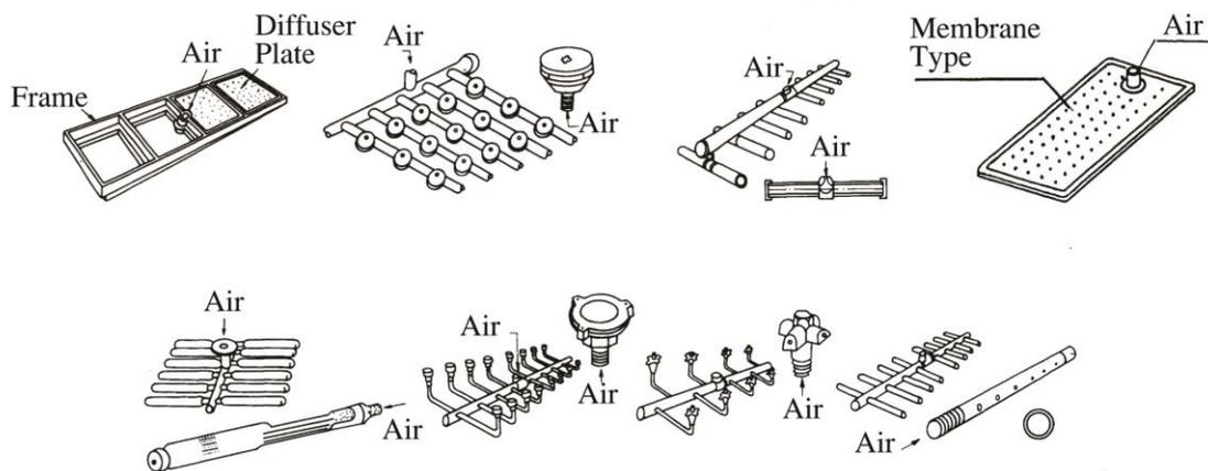
**Figure 5.9.1 Type of Diffuser**
