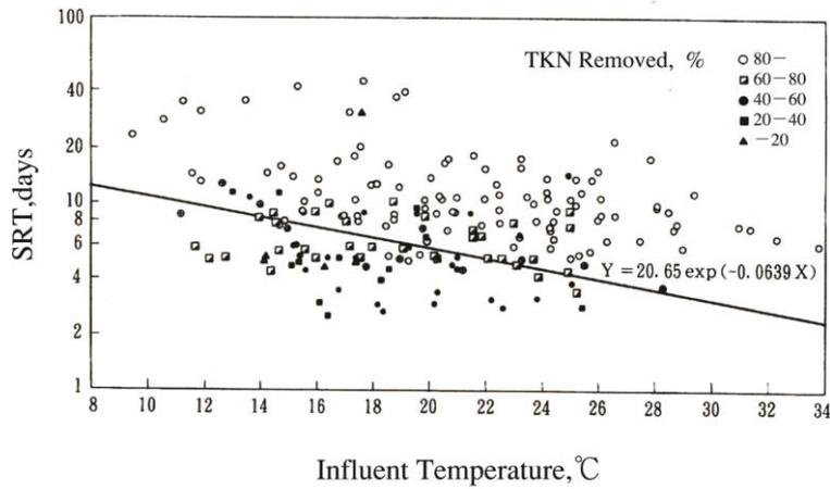
Figure 5.1.4 Necessary SRT for Nitrification and Influent Temp
