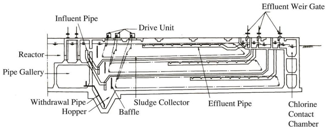
Figure 4.21.2 Three Tray Final Sedimentation at Osaka
