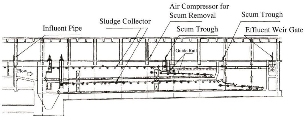
Figure 4.21.1 Two Tray Final Sedimentation at Kyoto
