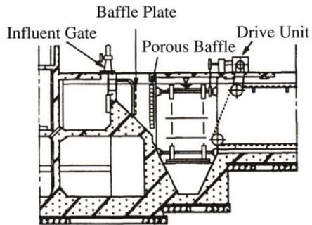
Figure 4.6.1 Inlet Structure
