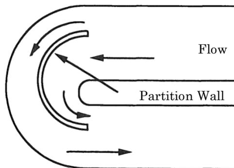
**Figure 5.20.1 Partition Wall for Flow Velocity Control**
