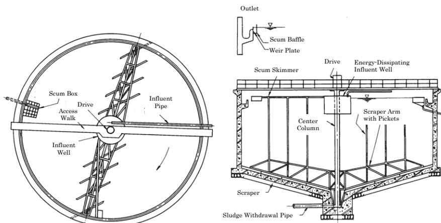
**Figure 5.24.1 Circular Center-Feed and Rim Take-Off Sedimentation**
