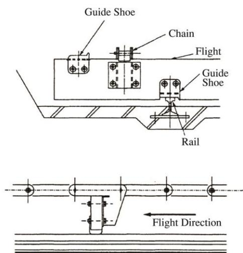
**Figure 4.9.1 Flight and Chain Sludge Collection, Diagram**
