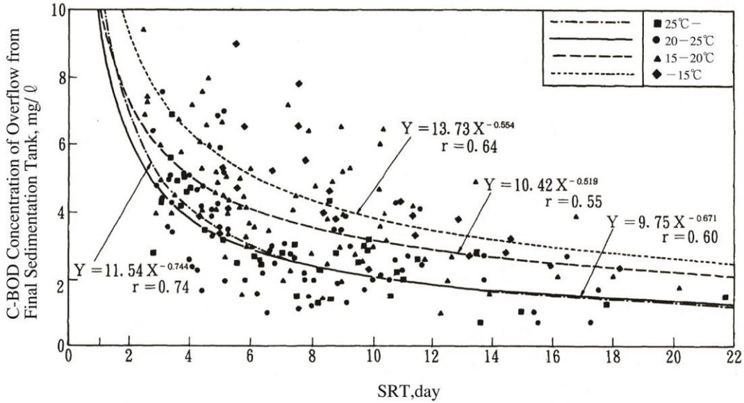
Figure 5.1.3 Effluent C-BOD and SRT at Operational WWTPs
