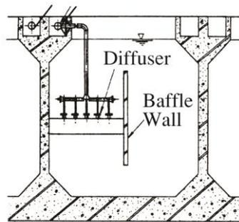
**Figure 5.6.2 Aeration System in Deep Aeration Tank**
