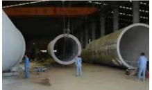
In april 2005, the interior of 22 wind mills of Zephyros in Taiwan has been treated with the Zingaceram system. This system has a life expectancy of > 15 years in a maritime zone with high humidity and aggressive environment.
