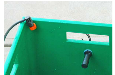
Position the adjustable control dripper so that it drips water into the evaporator
