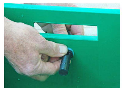
Install the float switch
