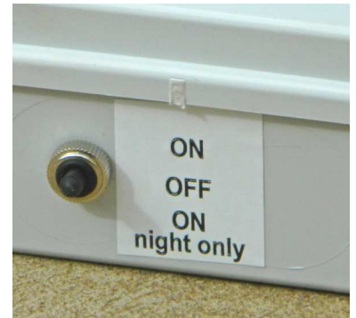
Switch with 3 positions: ON, OFF, ON night only
