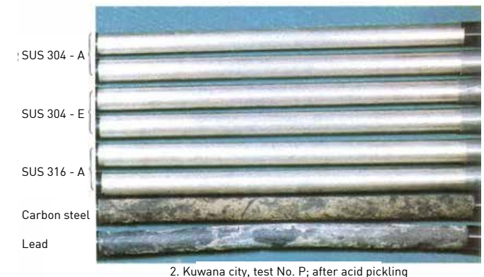
Photos of the burial test results after 10 years of burial in Kushiro (North-East Japan) and Kuwana (Central Japan).
