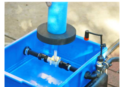
Slide the float over the float shaft
