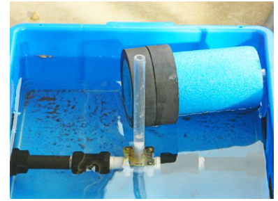
Remove the float to stop irrigating
