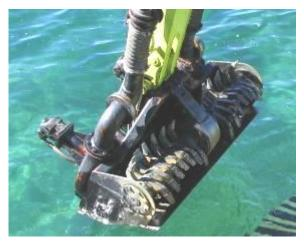
The Rake works like the standard bucket and it is used for removal of debris and vegetation.
