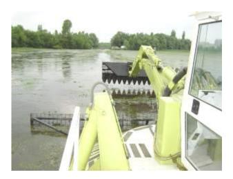
The Amphibex is equipped with a quick coupling system for attachments replacement.
