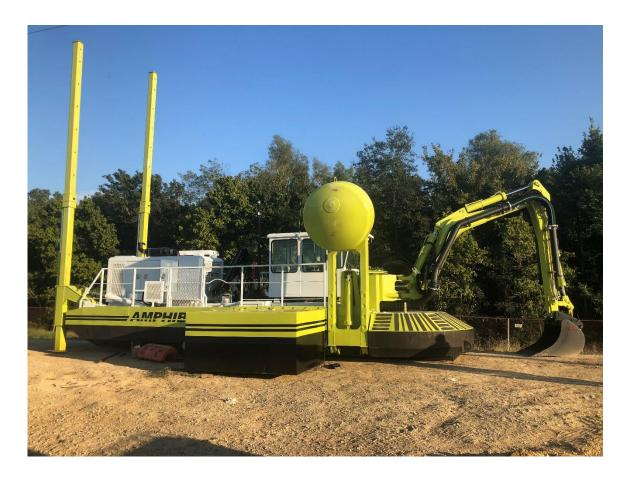
The maximum length of the machine is 11m, with an approximate working weight of 22 metric tons. Its approximate speed on water (with the propeller) is 5 to 8 knots.
