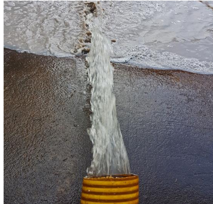
Abrimix treated water discharging back into the untreated wash bay waste water holding sump.
