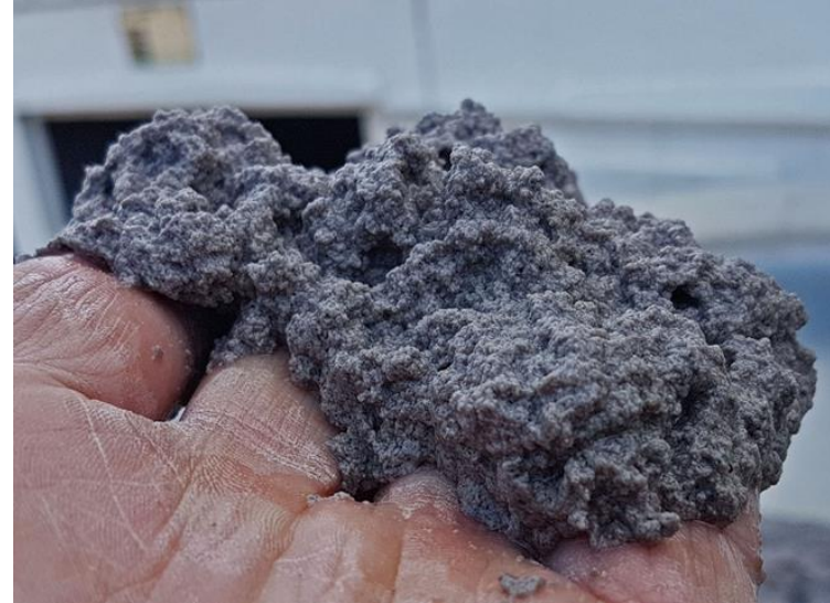
Separated solids held by hand to show reduced moisture content there of
