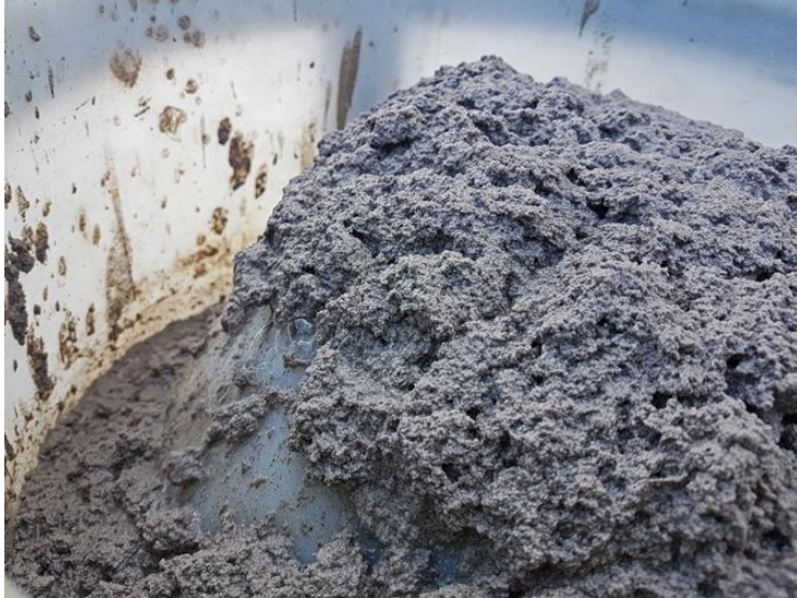
Separated solids discharging off the top of the SSF tank
