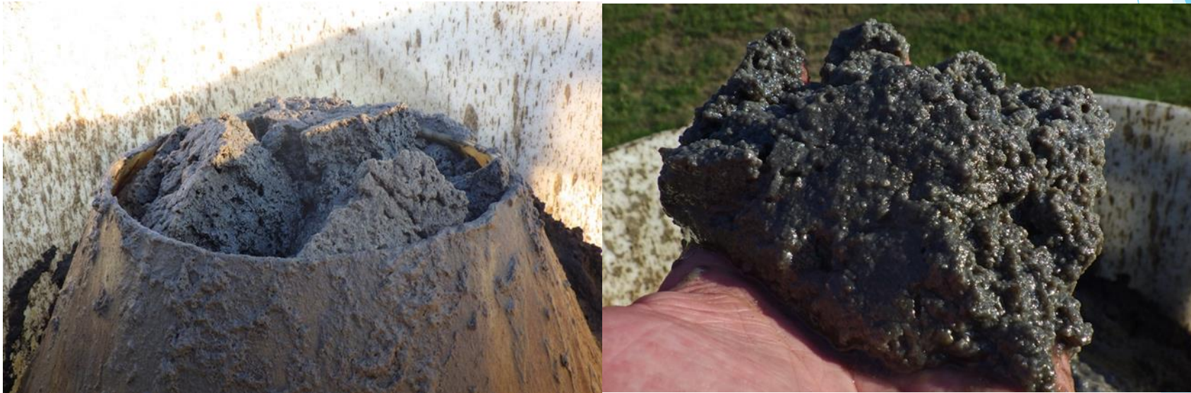
Separated oil & sludge from the waste discharge water stream
