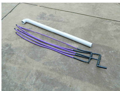
Dripper assembly for zone 8 with 15 8 lph drippers using Netafim Aries HWD 13 mm dripline
