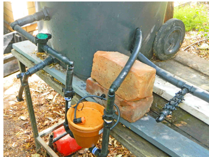
2. The outlet from the header tank delivers water to the inlet of an Unpowered Terracotta Irrigation Controller with the control dripper 20 cm below the header tank outlet. The outlet from the Unpowered Terracotta Irrigation Controller delivers water to a length of 25mm polypipe 20 cm below the header tank outlet.
