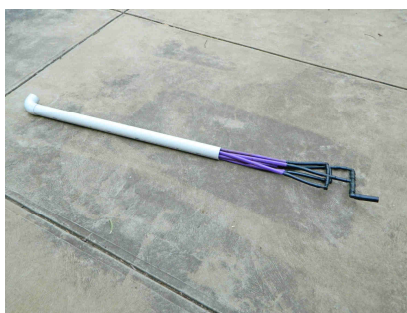
The dripper assembly is inserted inside an open pipe.
