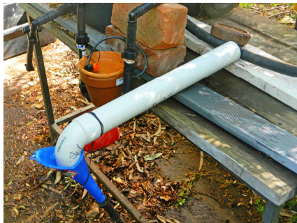
5. An open pipe collects the water from the dripper assembly and directs the water into a funnel.
