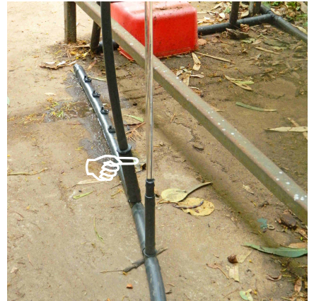
6. Polypipe delivers water from the funnel to the irrigation drippers. A clear vertical tube indicates a pressure of 35 cm head at the irrigation drippers.
