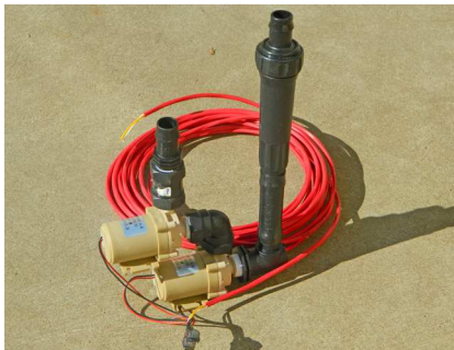
double pump (two pumps connected in series) with an inlet filter, fittings to connect to 19 mm poly pipe, and 9 metres of waterproof electrical cable
