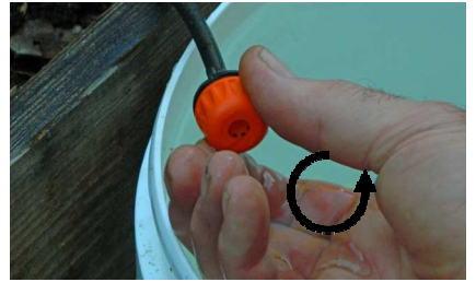
If the volume in the measuring container is more than the dripper control volume, turn the control dripper anticlockwise to increase the flow rate of the control dripper.
