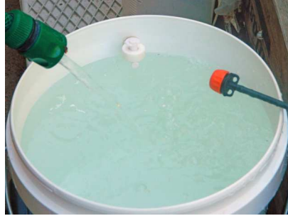
Fill the evaporator with water until the water level is just below the float switch
