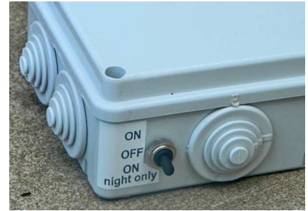
The switch on the irrigation controller has 3 positions: ON, OFF, ON night only
