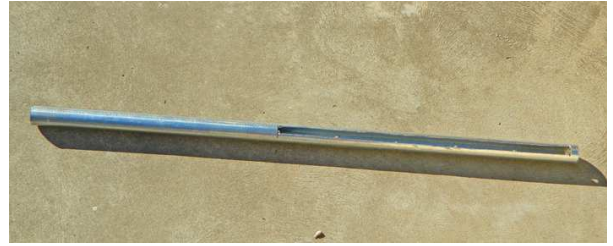
An angle grinder can be used to make a long slot in a length of steel pipe
