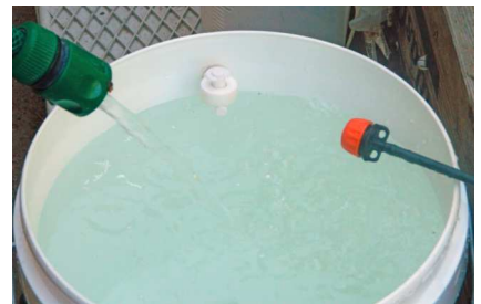
Fill the evaporator with water until the water level reaches the float switch
