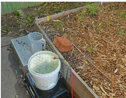
Evaporator, float switch and control dripper for zone 1
