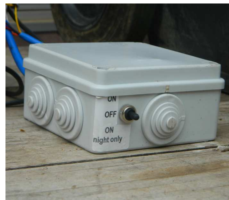
The switch on the irrigation controller has 3 positions
