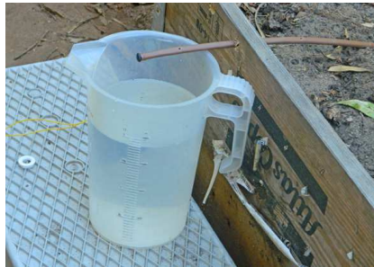
Dripper control volume in measuring container
