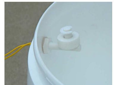
Float switch installed on evaporator with float shaft pointing up
