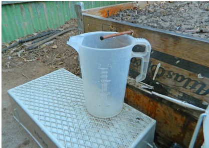
Place a measuring container under one of the irrigation drippers
