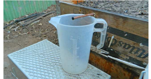
Measuring container under one of the irrigation drippers
