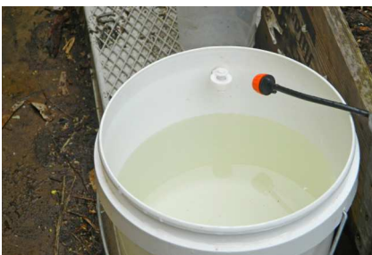
While the soil is drying, the water level in the evaporator is falling due to evaporation
