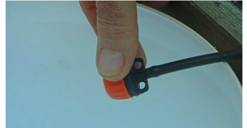
Adjust the control dripper so that flow rate is about the same as the flow rate of the irrigation drippers
