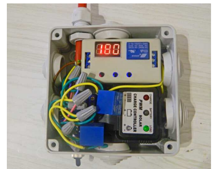
The delay timer has a 3 digit display for the time delay in seconds
