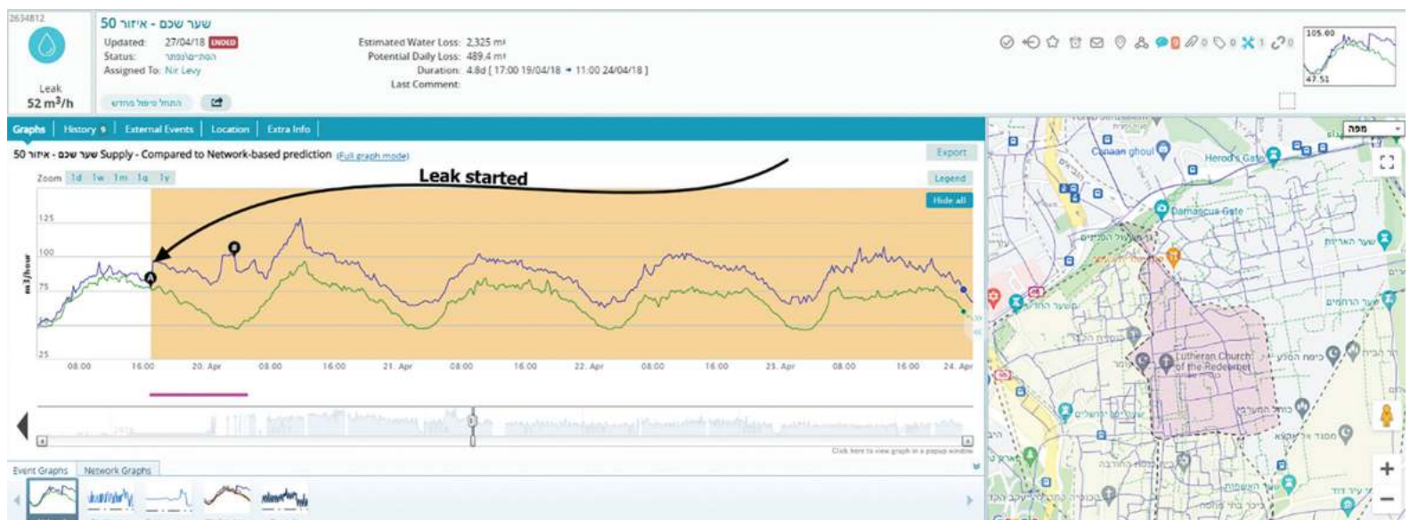
The TaKaDu Event Graph Shows Water Supply For The DMA. When The Leak Started It Is Easy To See The Wide Deviation Between The Predicted Behavior (Green) And The Actual Water Flow (Blue).
