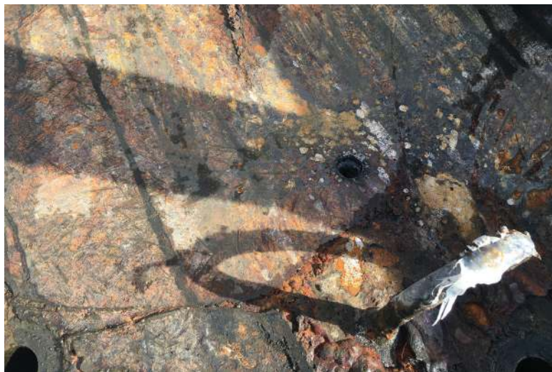
A One-Inch Hole Was Found To Be The Source Of The Leak On The 30-Inch Stub Out
