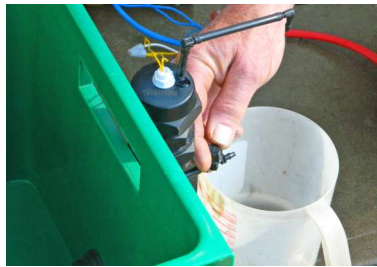
Close the 4mm valve on the float switch assembly
