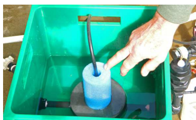
Push the float down to start irrigating
