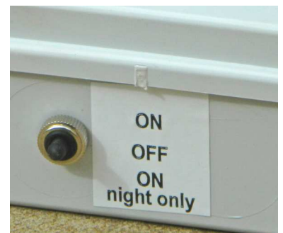
Switch with 3 positions: ON, OFF, ON night only
