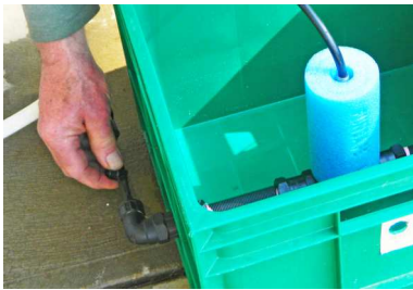
Close the 4mm valve on the inlet assembly
