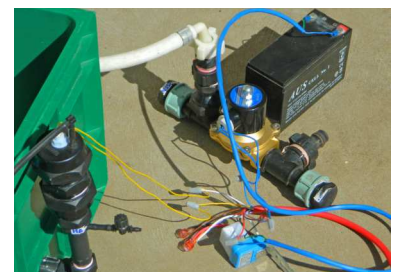
Connect the colour-coded wires from the control box to the float switch assembly, the solenoid valve and the power supply
