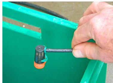
Position the adjustable control dripper so that it drips water into the evaporator
