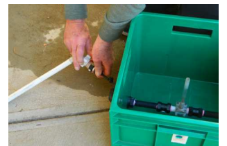
Connect the water supply to the inlet assembly
