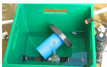
Remove the float to stop irrigating
