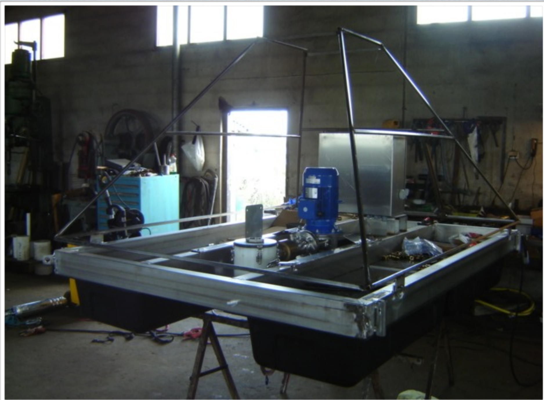
Production line: EffectiveNew™ 50m³/h placed on a raft
