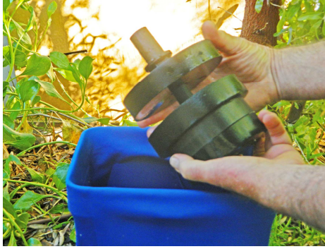
The adjustable gap between the upper and lower float determines the dripper discharge
