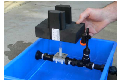
Slide the float over the float shaft
