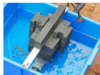
26mm net evaporation between irrigation events (20mm gap between magnet and bottom of full slides)
