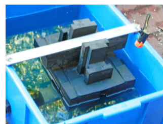
48mm net evaporation between irrigation events (20mm gap between magnet and bottom of cut slides)
