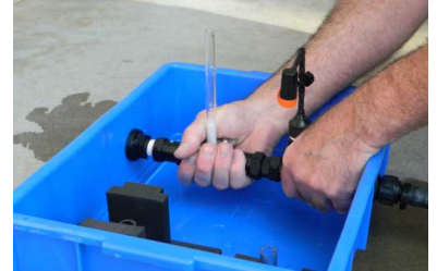
Float shaft must be vertical
