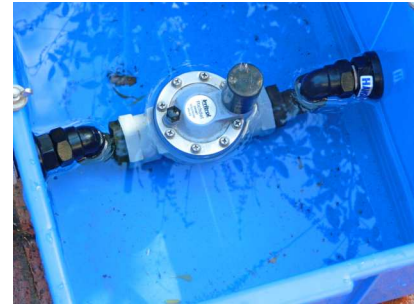
Unpowered Irritrol solenoid valve
