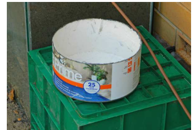
An evaporator with a surface area of 370 square cm
