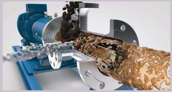
Veolia's patented thermal hydrolysis technologies are considered the next generation high solids thermal hydrolysis processes as they are able to process sludge directly from dewatering units, without any dilution (proven operation from 22% DS up to 32% DS in real world use), using the state-of-art dynamic mixers to instantaneously condense steam on to sludge.
