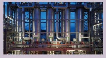
Veolia has, over the past 20 years, developed **Exelys™** and **BioThelys™**, two innovative high solids thermal hydrolysis solutions. While Exelys is a fully continuous process, Bio Thelys is a continuous batch process. Both processes utilize high temperature (310 to 330 oF) and pressure (85 to 100 PSIG) to sterilize sludge which is retained (SRT) for 20 to 30 minutes in a reactor at this elevated temperature and pressure.
