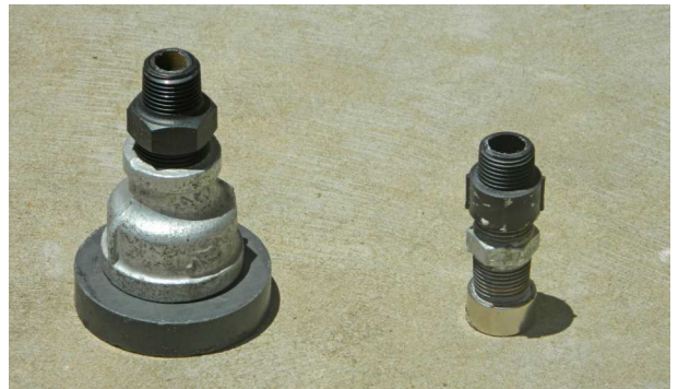
Ferrite ring magnet assembly on the left Rare earth disc magnet assembly on the right
