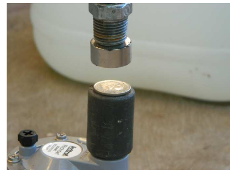
Spacer on top of the solenoid
