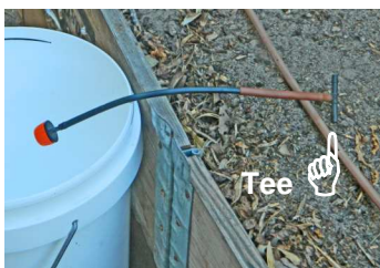
The adjustable dripper can be connected to a drip line using a Tee
