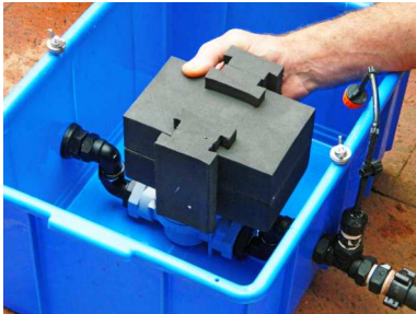
Position the float over the solenoid
