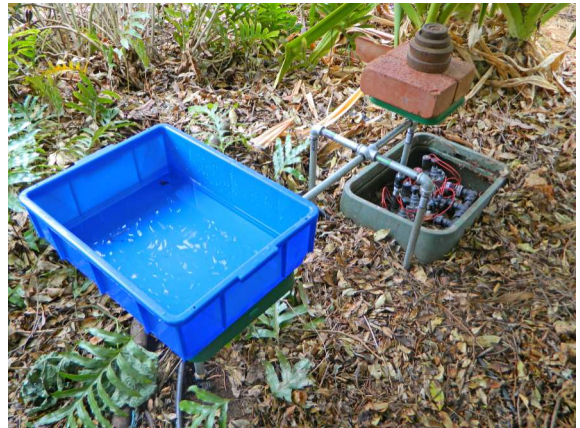
Add water to the evaporator until the depth is at least 20mm
