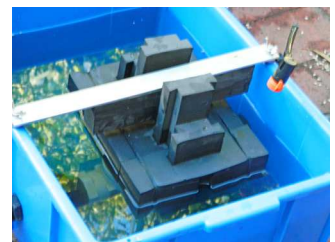
48mm net evaporation between irrigation events (20mm gap between magnet and bottom of cut slides)
