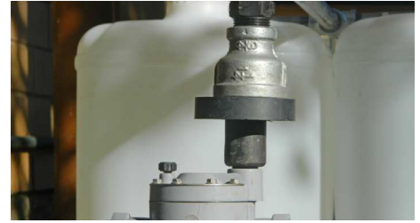
When the ferrite ring magnet assembly is in the high position, the top of the solenoid should be 10mm inside the ring magnet
