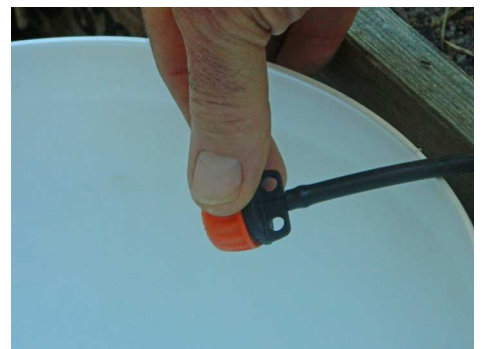
Adjust the control dripper so that flow rate is about the same as the flow rate of the irrigation drippers
