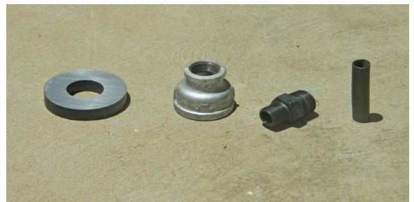
Components of the ferrite ring magnet assembly
