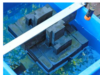
44mm net evaporation between irrigation events (15mm gap between magnet and bottom of cut slides)
