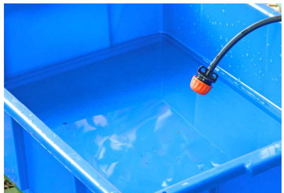
Position the adjustable dripper so that it will drip water into the evaporator
