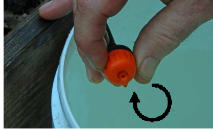
If volume in the measuring container is less than the dripper control volume, turn the control dripper clockwise to reduce the flow rate of the control dripper.
