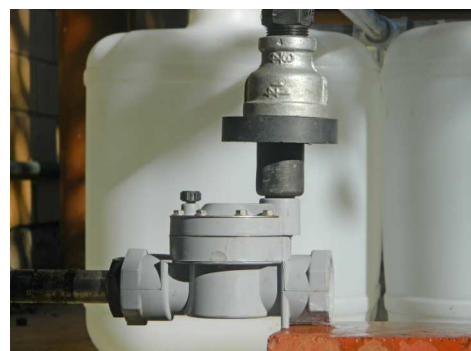
When the magnet is in the high position, the plunger is released and the valve closes
