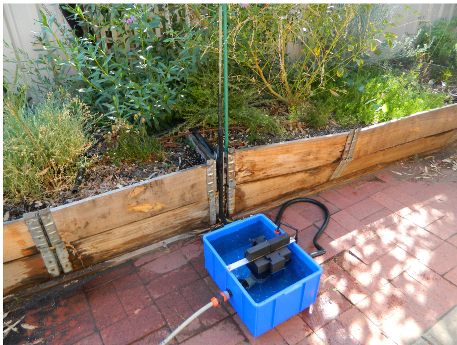
Hi-flow Unpowered Measured Irrigation Controller (HUMIC)
