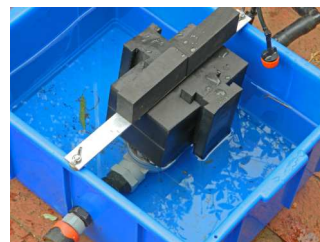
23mm net evaporation between irrigation events (zero gap between magnet and bottom of full slides)
