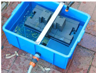
13mm net evaporation between irrigation events (zero gap between magnet and bottom of full slides)
