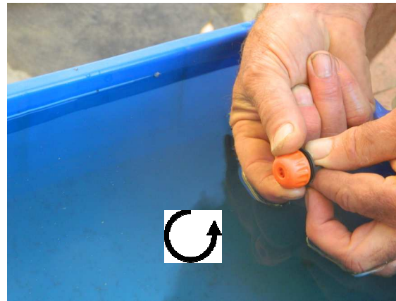
If you decide that your plants are getting too much water, then turn the control dripper anticlockwise to decrease the water usage.
