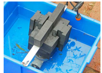
26mm net evaporation between irrigation events (20mm gap between magnet and bottom of full slides)
