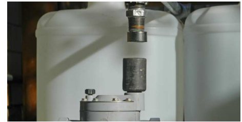
When the rare earth disc magnet assembly is in the high position, the top of the solenoid should be 20mm below the magnet
