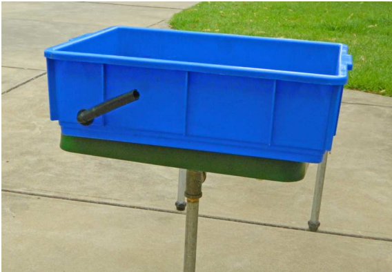
Rotate the elbow so that the end of the poly pipe is set at the desired overflow level
