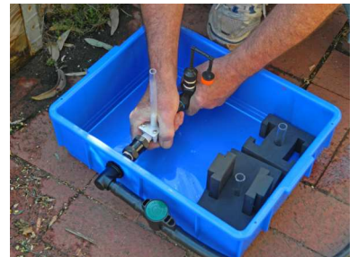
Float shaft must be vertical
