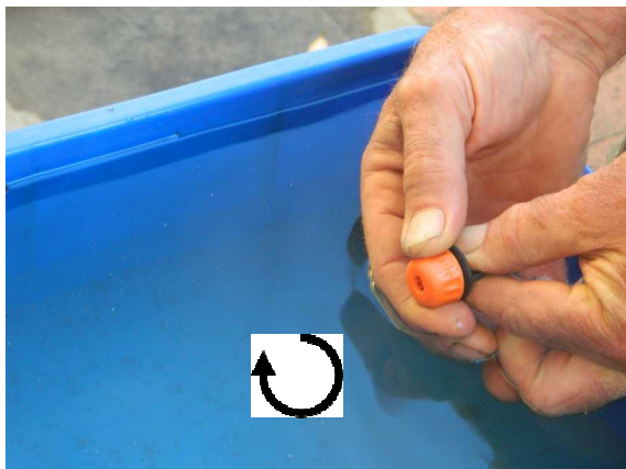
If you decide that your plants are not getting enough water, then turn the control dripper clockwise to increase the water usage.
