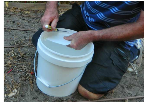
Draw a line on the inside of the evaporator about 1.5 cm below the overflow level
