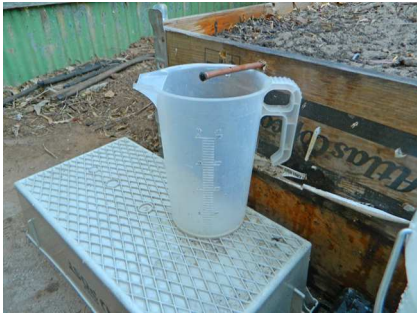
Place a measuring container under one of the irrigation drippers
