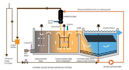
The ballasted material in the settling tank is pumped to the MA Hydrocyclone and the overflow of the Hydrocyclone is sent into the recirculation loop
