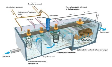
ACTIFLO Softening is designed to reduce Hardness, Alkalinity, Silica and Heavy Metals by addition of lime and/or Soda Ash.
