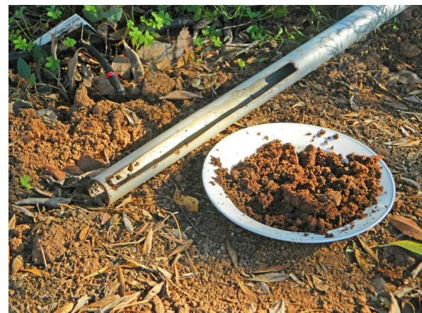
Measure the moisture content of the soil by weighing the moist soil, drying the soil in an oven, and then weighing the dry soil
