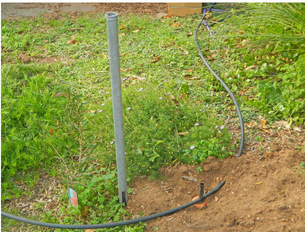
Use the soil moisture probe to measure the soil moisture content at various distances from the centre of the pitcher
