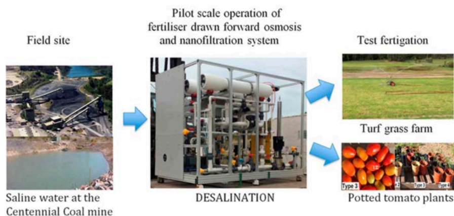
Figure 12-8 Pilot-scale of FDFO-NF hybrid system in Australia (Source: Phuntsho et al. , 2016)
