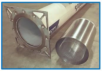
The Cyclone Reactor System is a flow through reactor engineered to release ready-state Water Lynx polymer into the water within the Cyclone chamber. The Cyclone chamber accelerates Water Lynx release utilizing induced vortex energy; this enables treatment of higher flow rates in a smaller footprint. Upon flow release from the Cyclone chamber, the flocculated solids aggregate based on reduced flow energy and induced cyclonic flow.
