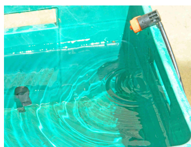
When the water level has fallen below the float switch, the irrigation starts automatically
