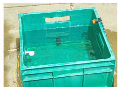
When the water level covers the float switch the irrigation stops automatically
