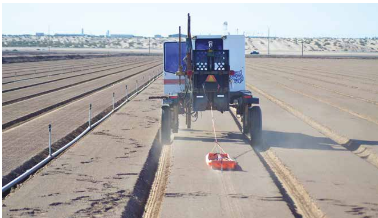
Figure 7. EM38 pre-plant conductance survey.
