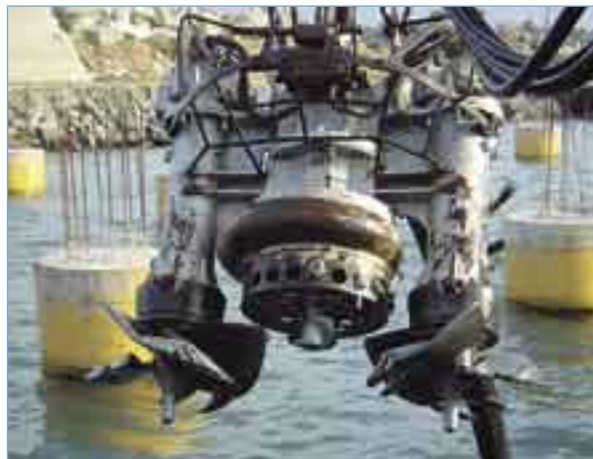
THY85A + 2 ExPro20: sea bed lowering at Gioiatauro Port (Italy).
