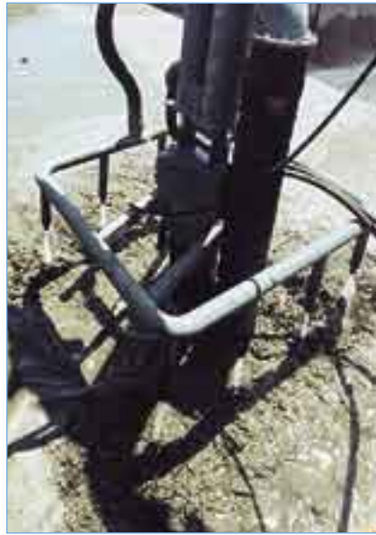
THY400: sand barge discharging (USA).
