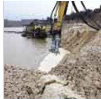
THY85B + 2 ExPro20: fixed on excavator boom for sand extraction (UK).
