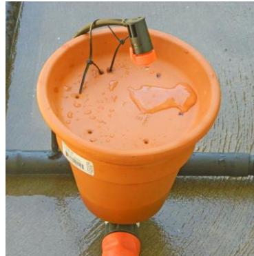
Place the terracotta saucer on the terracotta pot so that the control dripper drips water into the pot
