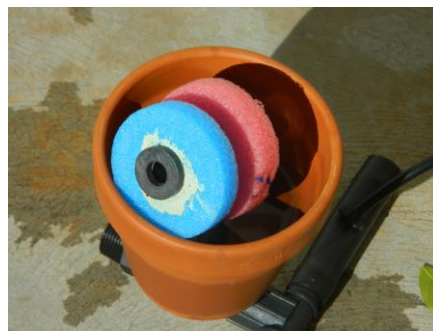
Float showing the ring magnet at the bottom of the float
