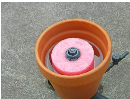
Unpowered Irrigation Controller showing the float the water level
