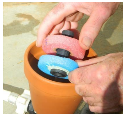
To adjust the interval between irrigation events, adjust the gap between the upper and lower float
