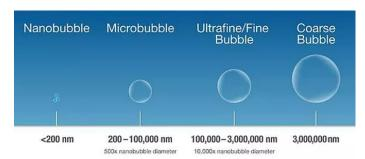
PRD Tech, Inc. has pioneered a unique gas stripping technology entitled "Controlled Nanobubble Stripping (CNS) process in which the stripping gas is dispersed in the aqueous phase, contaminated with the volatile chemical, in the form of nanobubbles, less than a micron in diameter. The interfacial surface area of nanobubbles is 400 times higher than for a 400 nm microbubble.
