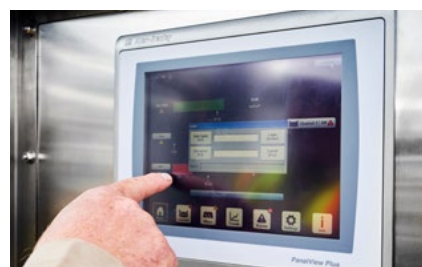
New controllers can be forward and backward compatible and feature large, color digital screens and intuitive icons.
