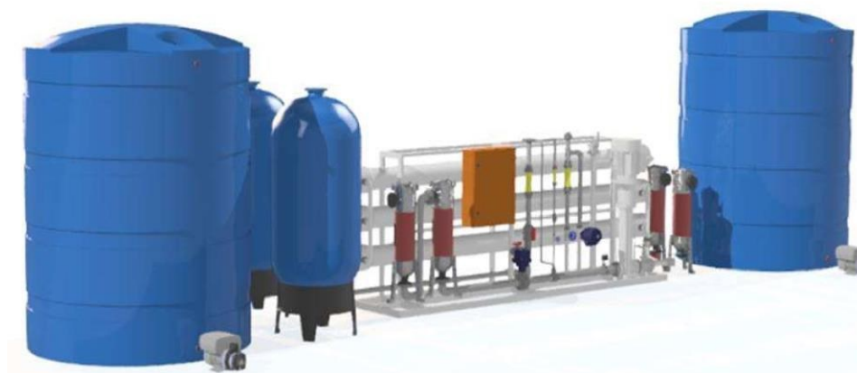
Figure 2 - Typical layout of AFM&RO plant
