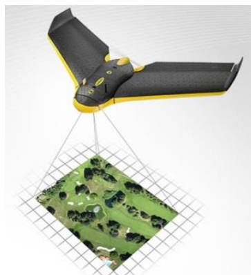
A drone (eBee from the Swiss company Sensefly) will be used for mapping at high resolution the studied shorelines.
