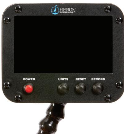
The versatile positioning arm, attached to the frame, offers an ergonomic solution for adjusting the **dipper-See Display Monitor** for viewing at different angles and lighting conditions. The monitor conveniently houses all of the controls on the front of the panel for ease of use. Recording the location, date, time and depth, will enhance the legitimacy of your findings and chain of custody.
