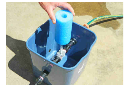
Slide the cylindrical float over the float shaft
