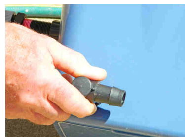
Inset the drain pipe into the drain hole in the bucket and reattach the elbow
