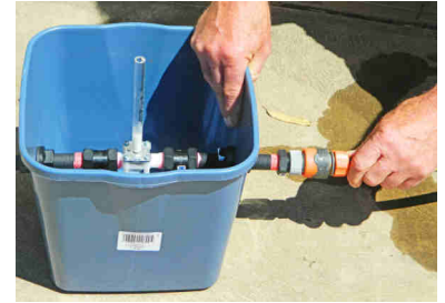
Connect the water supply to the inlet pipe on the bucket
