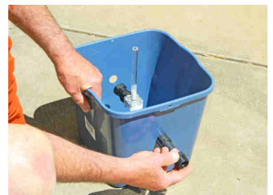
Reattach the round plastic nut and the inlet adaptor
