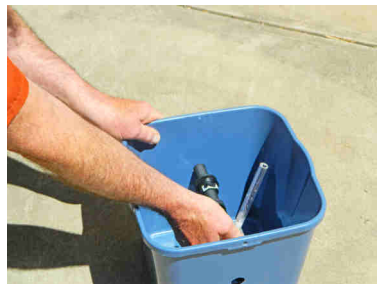
Insert the inlet pipe through one of the holes
