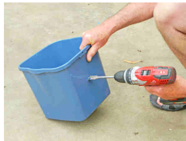
Drill 2 holes in opposite sides of the bucket
