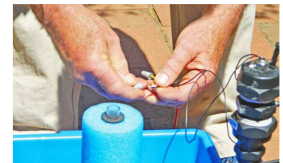
Connect the white and yellow wires to the Universal Measured Irrigation Controller
