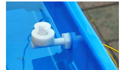
Irrigation starts automatically at the start time provided that the water level is below the float switch
