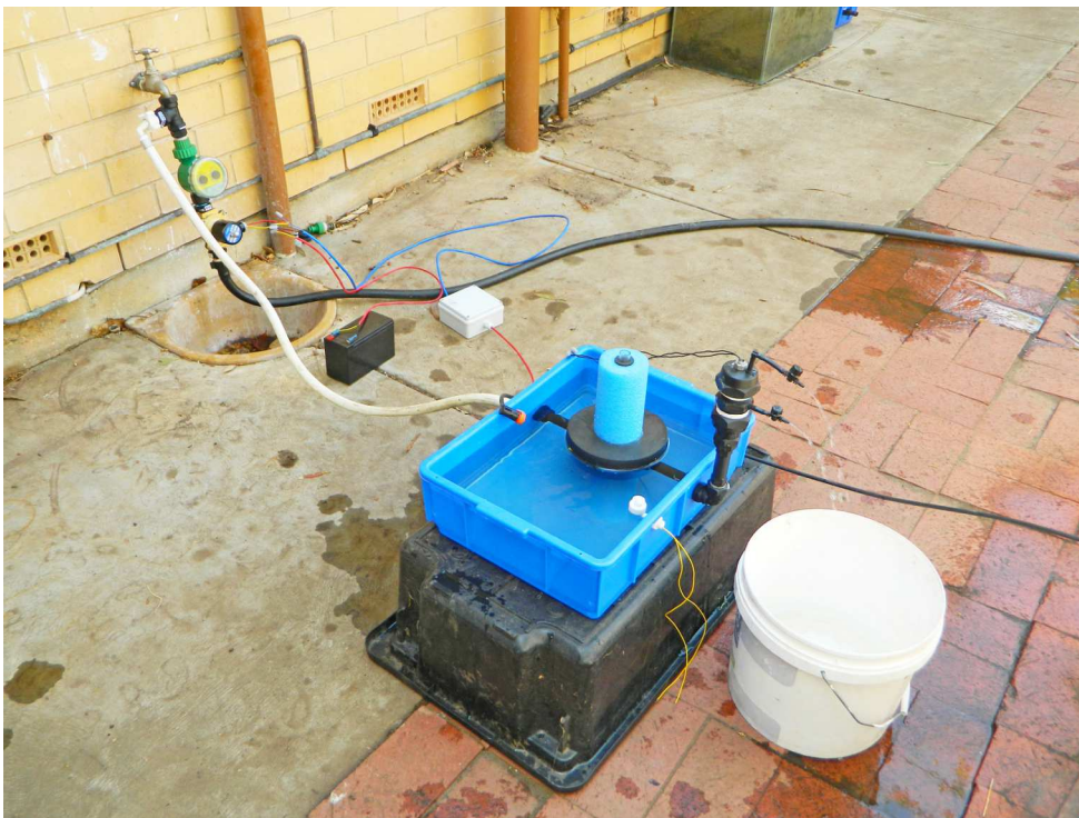
Universal Measured Irrigation Controller connected to a tap timer
