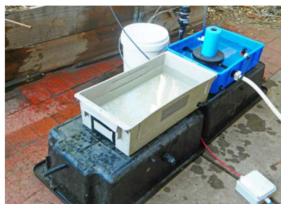
A supplementary evaporator increases the surface area of evaporation
