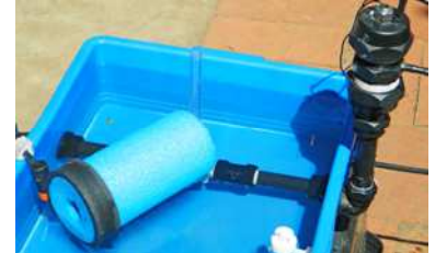
Remove the float to stop irrigating
