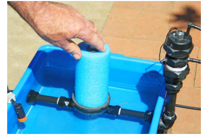
Push the float down to start irrigating
