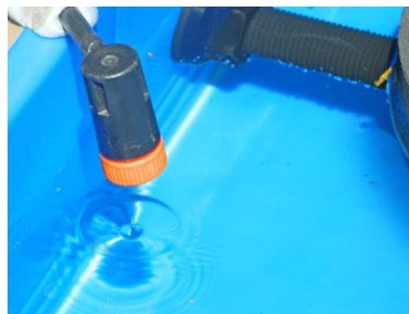
The control dripper drips water into the evaporator
