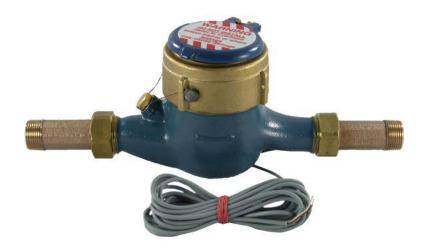
The MJR Series Pulse Meters offer pulse output from a reed switch sensor. This allows the two-wire contact type closure to operate metering pumps, remote indicators and controls.
